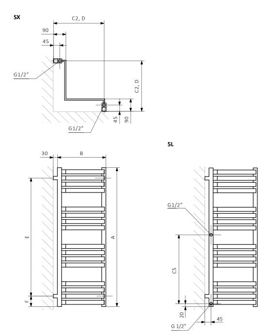
A - Height B - Width C1-C5 - Distance between pipe centres D - Horizontal distance between mounting bracket centres E - Vertical distance between mounting brackets F - Distance between a mounting bracket and the bottom of the radiator
