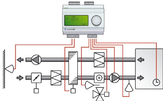
For control mode "Supply air temperature control with outdoor compensation" you need two sensors, "Supply air sensor" on AI1 and "Outdoor sensor" on AI2.
