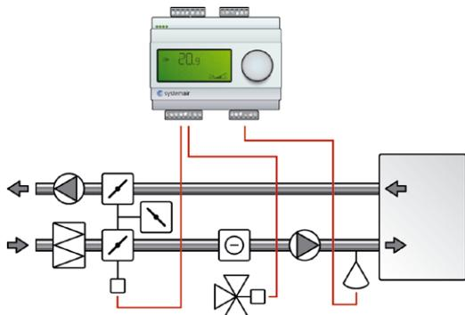
For control mode "Supply air temperature control" you need only one sensor, "Supply air sensor" on AI1
