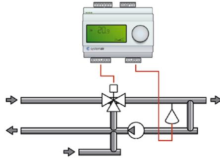
For this control mode you need a single sensor, “Supply water temperature” on AI1
