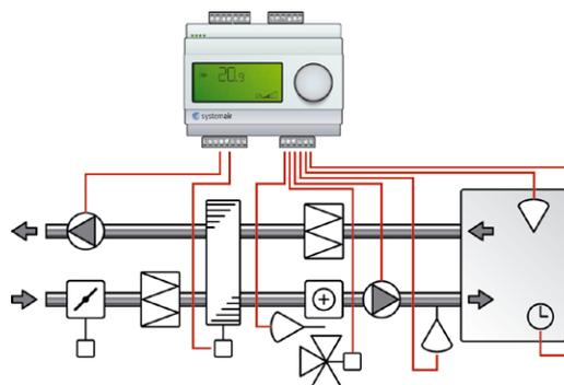
For control mode 3, "Cascade connected room / Exhaust air temperature control" you also need 2 sensors, "Supply air sensor" on AI1 and either "Room sensor" or "Exhaust sensor" on AI2.
