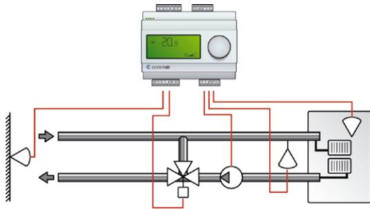
For this control mode you need two sensors, GT1 “Supply temperature” on AI1 and GT2 “Outdoor sensor” on AI2.
