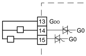
In OP10-230 however, the internal transformer's capacity restricts the current on  $G_{DO}$  to approx. 165 mA.
