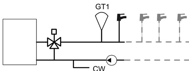
For this control mode you need a single sensor, “Supply water temperature” on AI1
