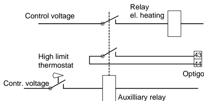
Wiring suggestion for high temp limit when using electric heating. Drawn with high temp limit activated.
