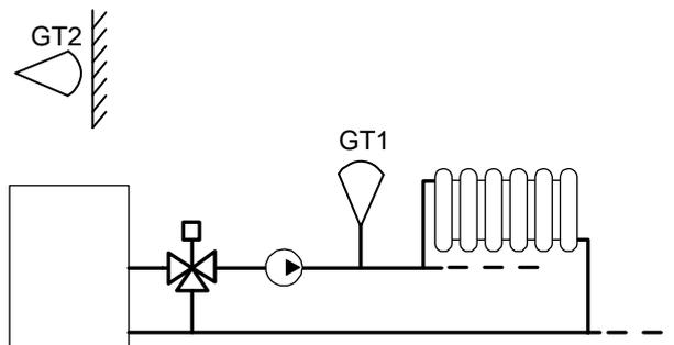
For this control mode you need two sensors, GT1 “Supply temperature” on AI1 and GT2 “Outdoor sensor” on AI2.
