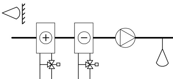
For control mode 3, “Cascade connected room / extract air temperature control” you also need 2 sensors, “Supply air sensor” on AI1 and either “Room sensor” or “Extract sensor” on AI2.
