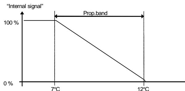
The frost protection signal (“Internal signal”) will increase linearly to 100 % at 7°C at which point the frost protection alarm is triggered. The fan will then be shut down and the controller will go into shutdown mode.
