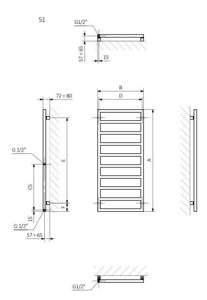
A - Height B - Width C1-C5 - Distance between pipe centres D - Horizontal distance between mounting bracket centres E - Vertical distance between mounting brackets F - Distance between a mounting bracket and the bottom of the radiator
