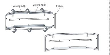
5. Reassembly the air inlet grille by reverse process of 1.
