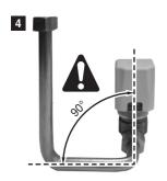
Make sure the piping is connected to the 2-way valve under a right angle, otherwise further installation becomes impossible.
