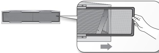
2. Clean the Air filter with a vacuum cleaner or soft brush. If dust is too heavy, then rinse it with running water and dry it in a ventilated area.
