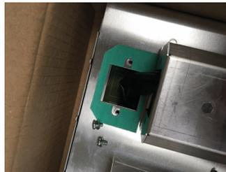
Stand the first leg up and remove the two Cover Screws holding the front cover on.
