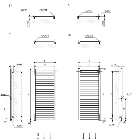
A - Height B - Width C1-C5 - Distance between pipe centres D - Horizontal distance between mounting bracket centres E - Vertical distance between mounting brackets F - Distance between a mounting bracket and the bottom of the radiator
