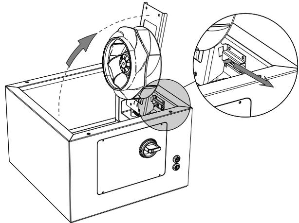
Lift the motor up by holding the motor bracket's handle, keep fingers away from the back of the hinge. Make sure that the motor bracket attach to the lock to prevent the motor from falling down during maintenance. After maintenance, release the lock, using the handle to bring the motor down. Fasten the motor bracket with the screws.
