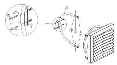
The bracket unit consists of: 1. ARM (1 piece); 2. HOLDER; 3. M8x60mm SCREW WITH A WASHER AND NUT FASTENING THE CLAMP (2 sets); 4. M8x60mm SCREW FASTENING THE HOLDER TO THE UNIT HEATER (2 pieces); 5. PLUG (2 pieces); 6. MOUNTING SLEEVE (2 pieces)
