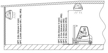
distance between units - recommended distance 6-12m (Volcano VR1, VR2, VR3), 3-7m (Volcano VR Mini), in order to ensure even hot air diffusion
