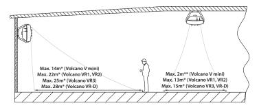
\* for horizontal air guide adjustment \*\* for symmetric air guide adjustment at an angle of 45°
